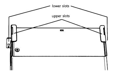
There are four corresponding tabs on the inside back panel of the computer which fit into the openings in the subassembly slots.
